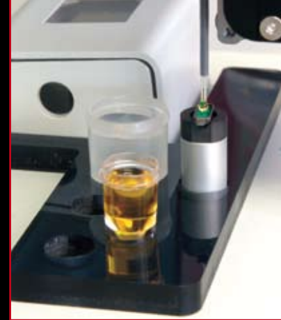
▲ Liquid dosing unit for SSA 600 – for automated calibration with liquid standards and addition of modifiers
